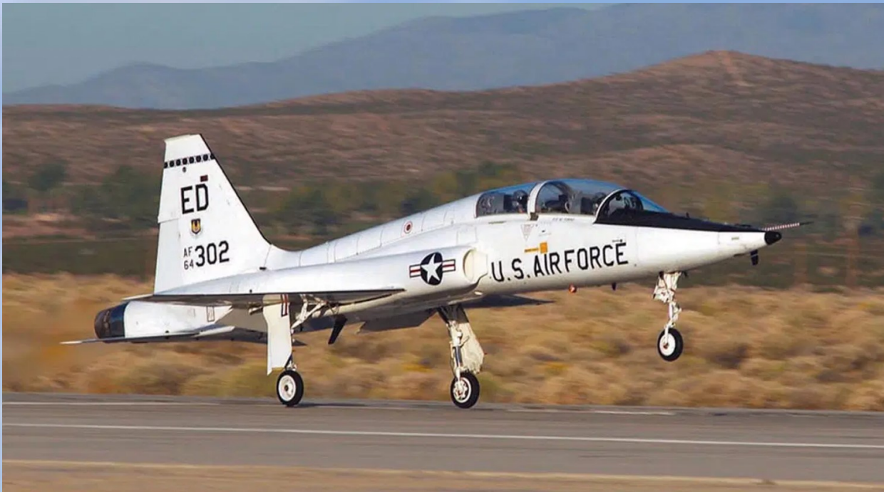
Northrop T-38 Talon: two-seat, twinjet supersonic jet trainer, First Maiden Flight (67 years ago the month) 10 April 1959
